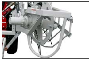
HYD. MOTORS MOUNT TO A HEAVY-DUTY BEARING HOUSING
