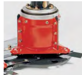
Direct drive of the cutter bar
