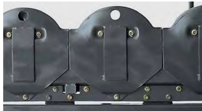
Fully protected cutter bar bottom
