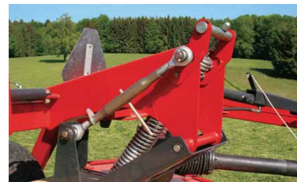
Setting the cutting height
