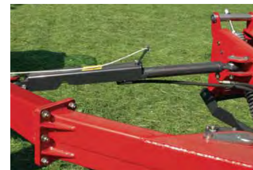
Displacement cylinder mechanically locked in working and transport position
