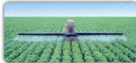
Air-Assist Boom System On
